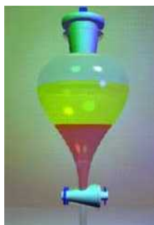
Figure.2.1. Separatory funnel used for extraction of solute
